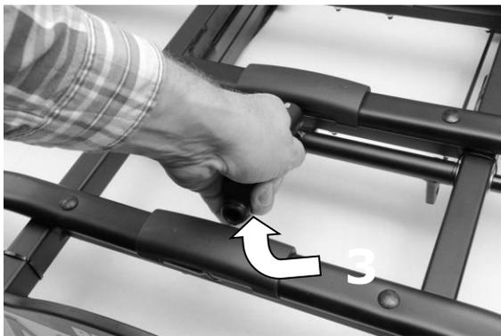
With one hand, keep a firm grip on the U-frame or bikes so that the carrier cannot fall down in an uncontrolled movement. With the other hand, pull the handle of the tilting mechanism up to unlock it (3). It is now possible to tilt the carrier.
